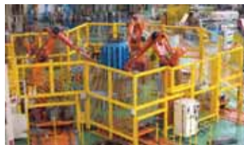
Robotic Stator Core Lamination Stacking
