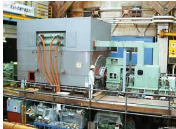
53 MW Synchronous Motor
